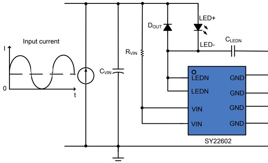
Figure 1. Schematic Diagram
