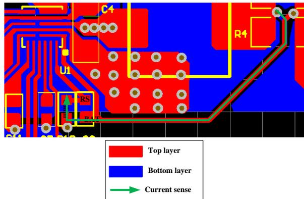
Figure 3. PCB Layout Suggestion
