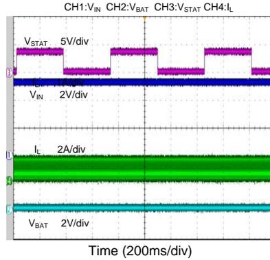
Steady Waveform When No Battery
