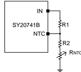
Figure 4. UTP /OTP configuration using  $R_1$  and  $R_2$
