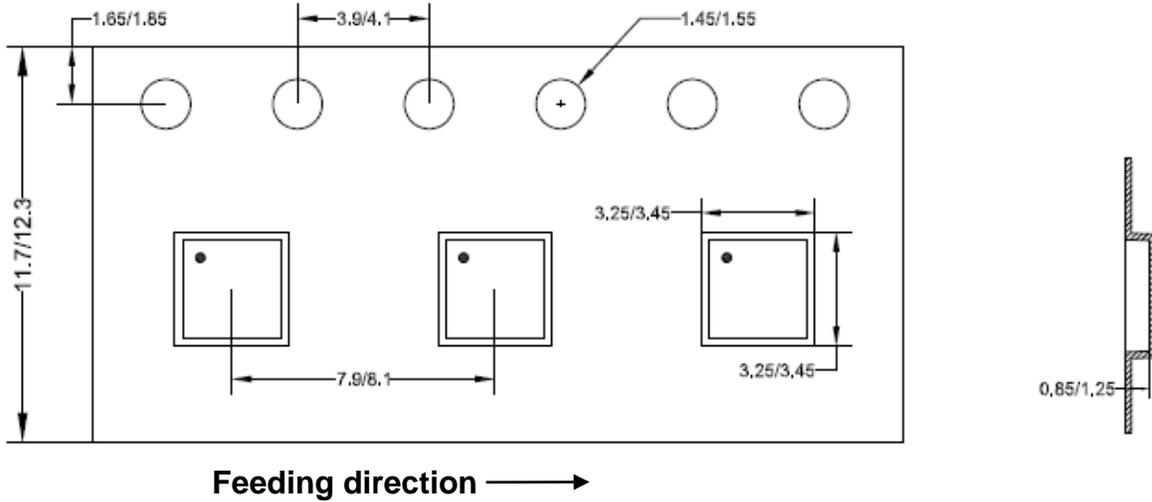
**Carrier Tape & Reel Specification for Packages**
