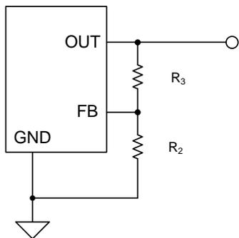
Choose R2 and R3 to configure the output voltage. Choosing large resistance values for both R2 and R3 is recommended to minimize power consumption under light loads. A value of between 1kΩ and 1MΩ is highly recommended for both resistors.
