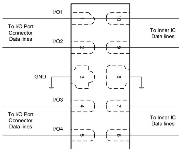
**Figure 2. SY205227DVD Pin Connections in PCB**
