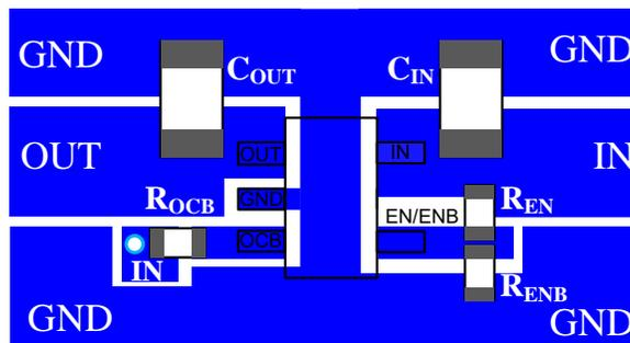
Figure 2. PCB Layout Suggestion
