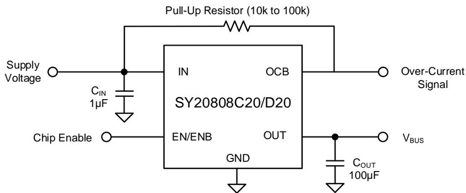
Note: If 1 $\mu$ F input cap will lead to large  $V_{in}$  voltage spike, it is strongly recommended to add additional 10 $\mu$ F ceramic cap.
