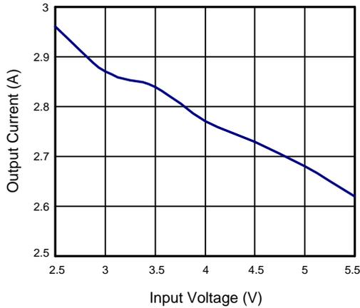
Current Limit vs. Output Voltage
