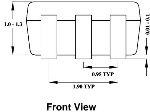
Note: All dimensions are in millimeters and exclude mold flash and metal burr.
