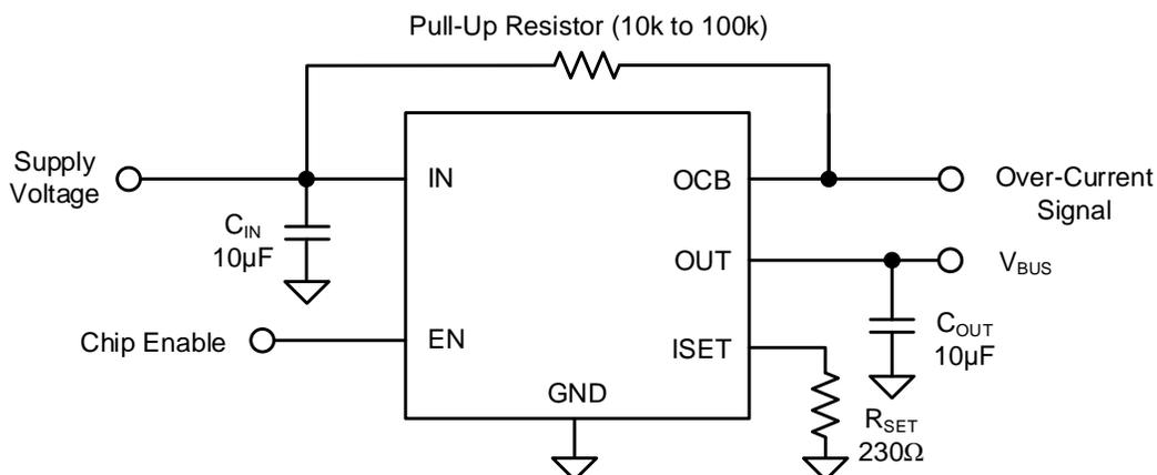
Figure 1. Schematic Diagram
