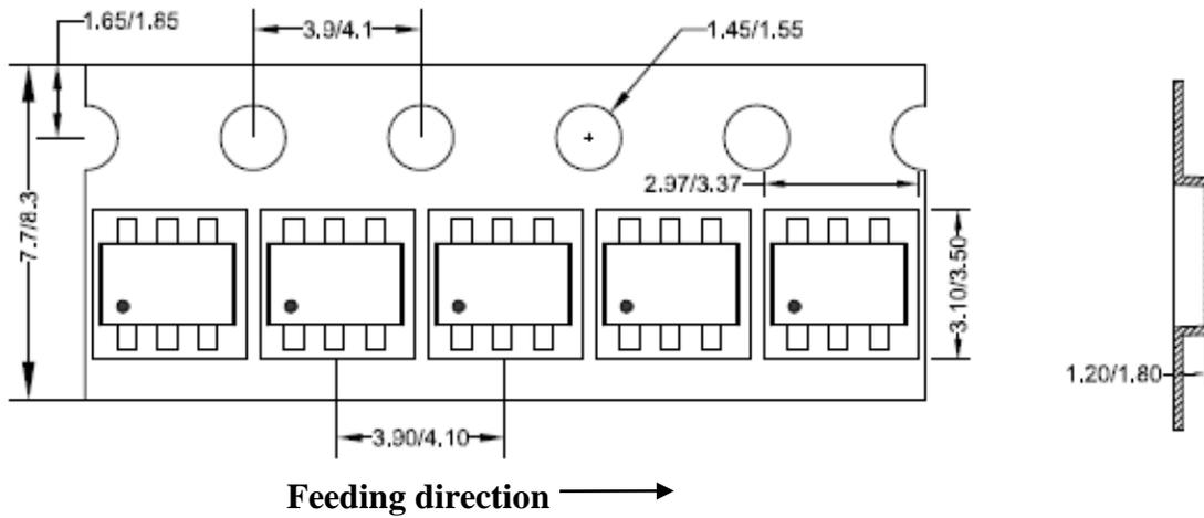
**2. Carrier Tape & Reel Specification for Packages**
