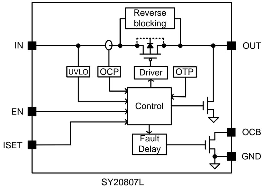
Figure 2. Block Diagram
