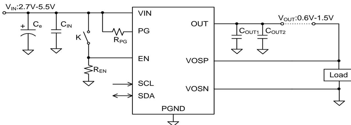
Figure 1. Schematic Diagram
