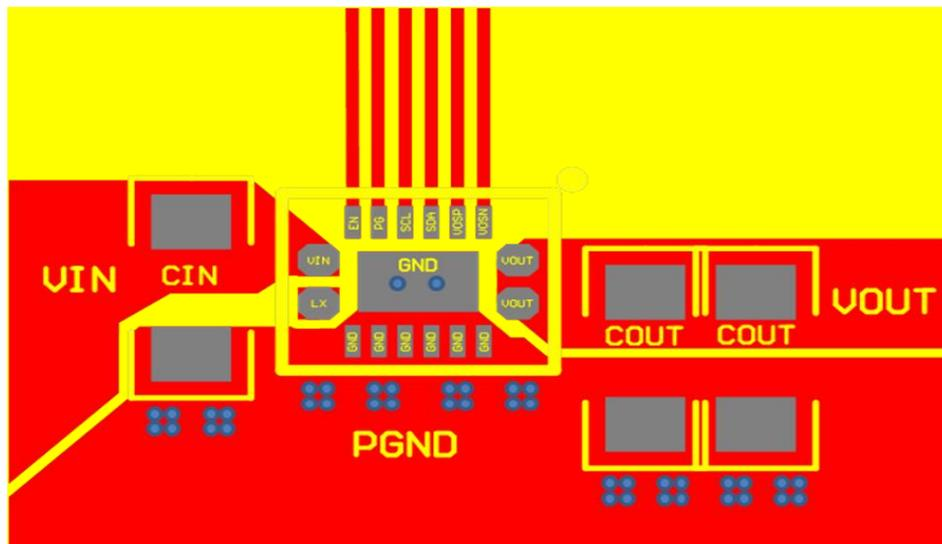
Figure3.PCB Layout Suggestion
