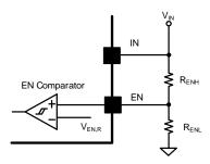
If the input UVLO threshold is low for some high input UVLO threshold requirement applications, use EN to adjust the input UVLO by adopting two external divided resistors.
