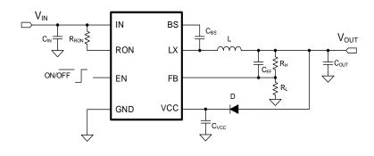
Figure 1. Typical Application Circuit
