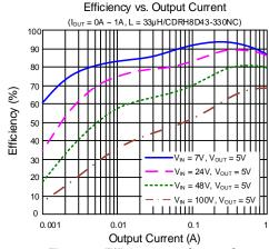
Figure 2. Efficiency vs. Output Current
