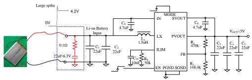
Figure 5. Voltage Spike Suppression
