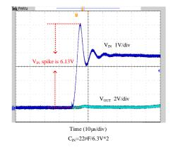
Figure 6. Voltage Spike without Suppression
