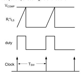
Figure 3. Constant-On-Time Peak-Current Control
