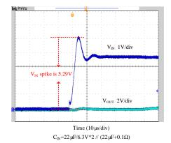
Figure 7. Voltage Spike with Suppression
