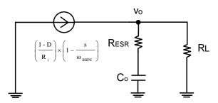
Figure 8. Current Feedback Loop
