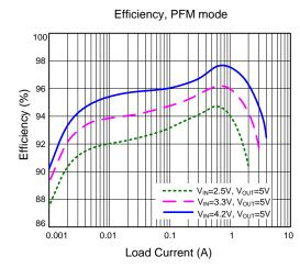
Figure 2. Efficiency vs. Load Current
