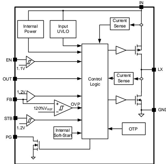
Figure 3. Block Diagram
