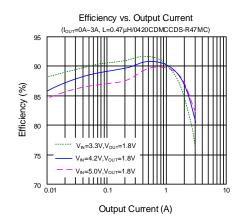
Figure 2. Efficiency vs. Output Current
