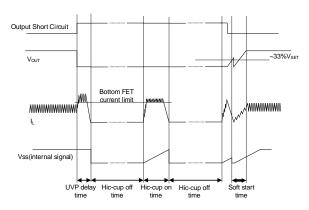
Figure 8. Output Undervoltage Protection
