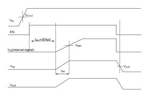
Figure 6. Startup and Shutdown Sequence
