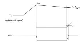
Figure 9. Overtemperature Protection
