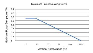
Figure 12. Maximum Power Dissipation
