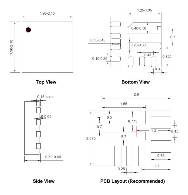
Notes: 1. All dimensions are in millimeters and exclude mold flash and metal burr. 2: The center of the PCB diagram refers to the chip center.
