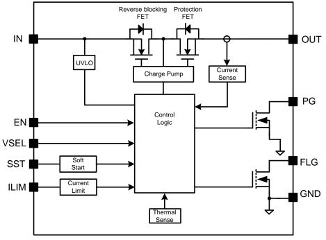
Figure 3. Block Diagram
