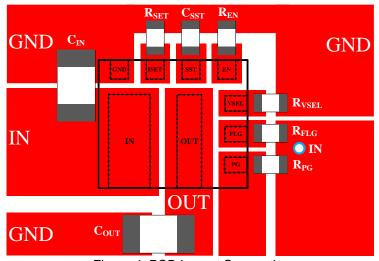
Figure 4. PCB Layout Suggestion
