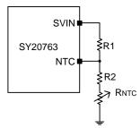
Figure 2. UTP /OTP configuration using R1 and R2
