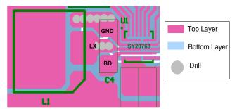
Figure 3. PCB Layout Suggestion
