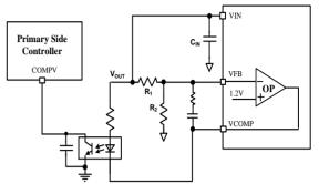
Figure6. DC Output Feedback Application Circuit
