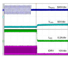
Power OFF ( $V_{IN(AC)}$ =220V) ( $V_{OUT}$ =12V,  $I_{OUT}$ =3A,  $V_{LED}$ =80V,  $I_{LED}$ =300mA)
