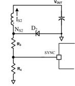
**Figure5. SYNC Application Circuit**
