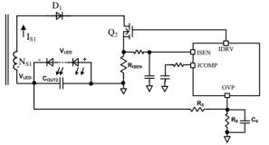
Figure 7. LED Open/Short Protection Application Circuit
