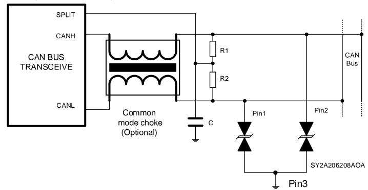
Figure 2. CAN Bus ESD/Surge Protection Circuit
