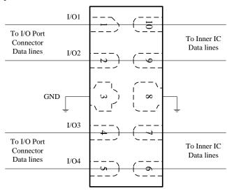
Figure 1. SYT06U05DVC pin connection in PCB
