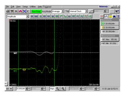
Figure 8. TDR Measurements for HDMI
