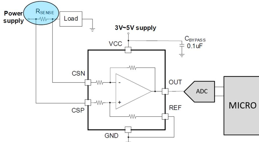
A range of Bi-Directional Current Sense Amplifiers for Precise Current Shunt Monitoring located either Low-side or High-side, with Low Quiescent Current (110uA[max]), in compact SOT363(SC70) packages.
