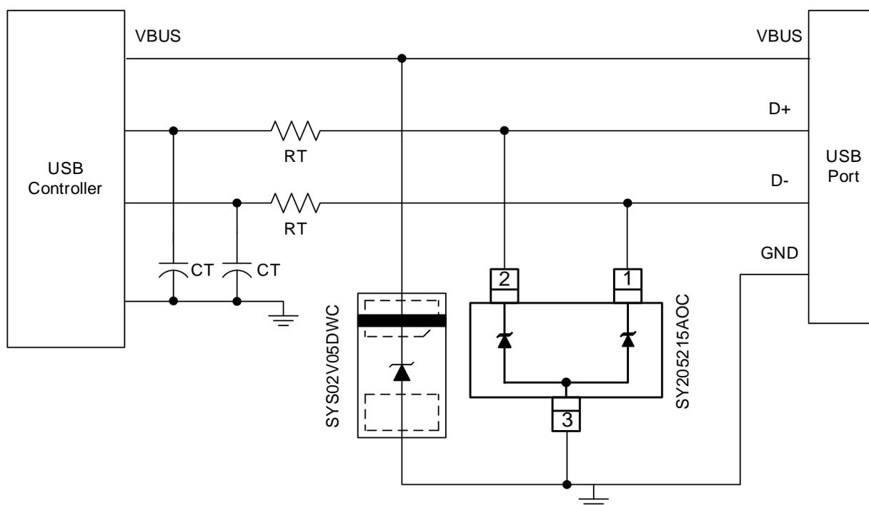
Figure 2. Typical ESD Protection for USB 2.0
