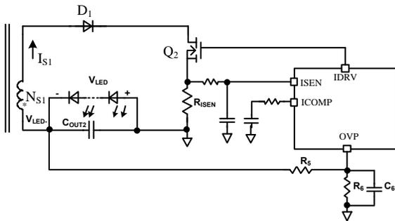
**Figure7. LED Open/Short Protection Application Circuit**
