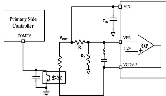
**Figure6. DC Output Feedback Application Circuit**
