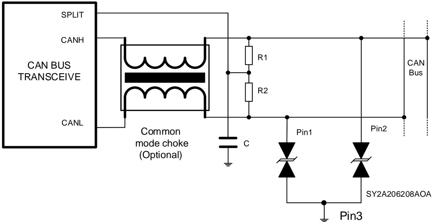
Figure 2. CAN Bus ESD/ Surge Protection Circuit
