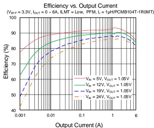
Figure 2. Buck Efficiency vs. Output Current
