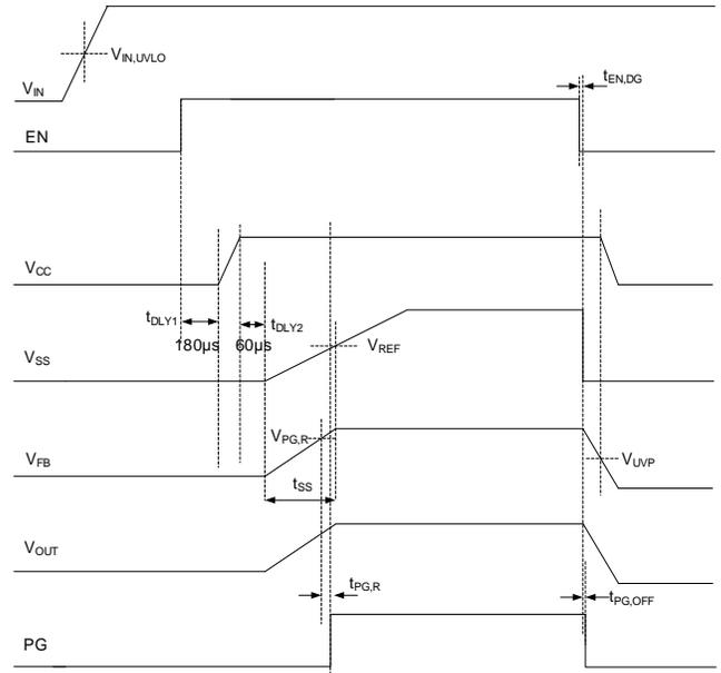
After  $V_{IN}$  exceeds the UVLO rising threshold, the VCC is turned on after the delay time  $t_{DLY1}$  if EN is high, the buck converter is turned on after another delay time  $t_{DLY2}$  after VCC voltage is set up. When the output voltage is 90% of the regulated value, PG is set to the high-impedance state after the delay time  $t_{PG,R}$ .
