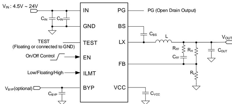
Figure 1. Schematic Diagram
