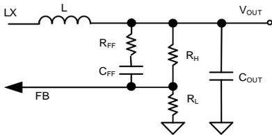
Note: For  $C_{OUT} > 500\mu F$  and when the minimum load current is low, use feedforward values of  $R_{FF} = 1k\Omega$  and  $C_{FF} = 2.2nF$  to provide sufficient ripple to FB node for low output ripple and good transient behavior.
