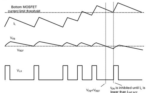
The device supports programmable valley current limit threshold. Pull ILMT pin low, floating or high for 3 gears successively increasing valley current limit threshold. When the valley current limit occurs, the output current limit value is
