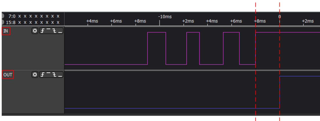
Figure 13-8. CNT/DLY Output in Rising Mode
