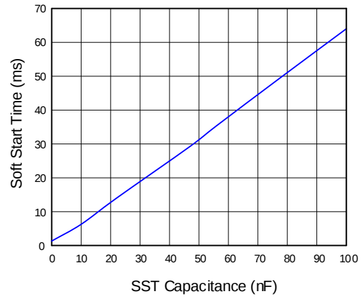
Soft Start Time vs. SST Capacitance ( V_{IN}=12V , No Load)
