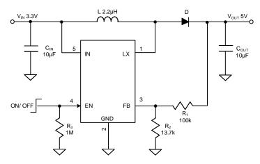
Figure 1. Typical Application Circuit
