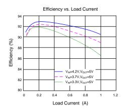
Figure 2. Efficiency vs. Output Current
