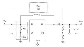
Figure 3. Inrush Current Limiting
