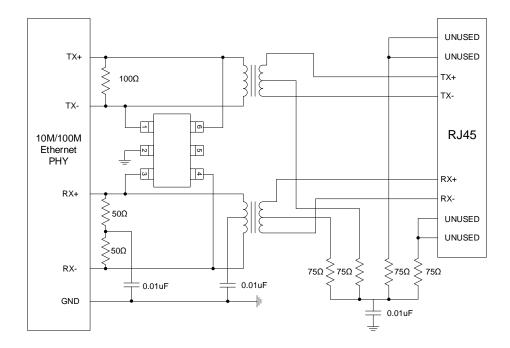
Differential and Common Mode Protection for 10M/100M Ethernet Interface with SY205236ABC
