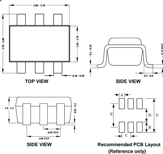
Note: All dimensions are in millimeters and exclude mold flash and metal burr.
