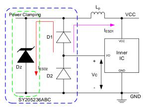
Figure 3. Positive ESD Clamping Voltage Optimization
