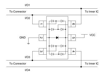
Figure 2. SY205236ABC Pin Connection in PCB
