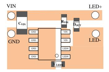
Figure 4. Recommend PCB Layout
