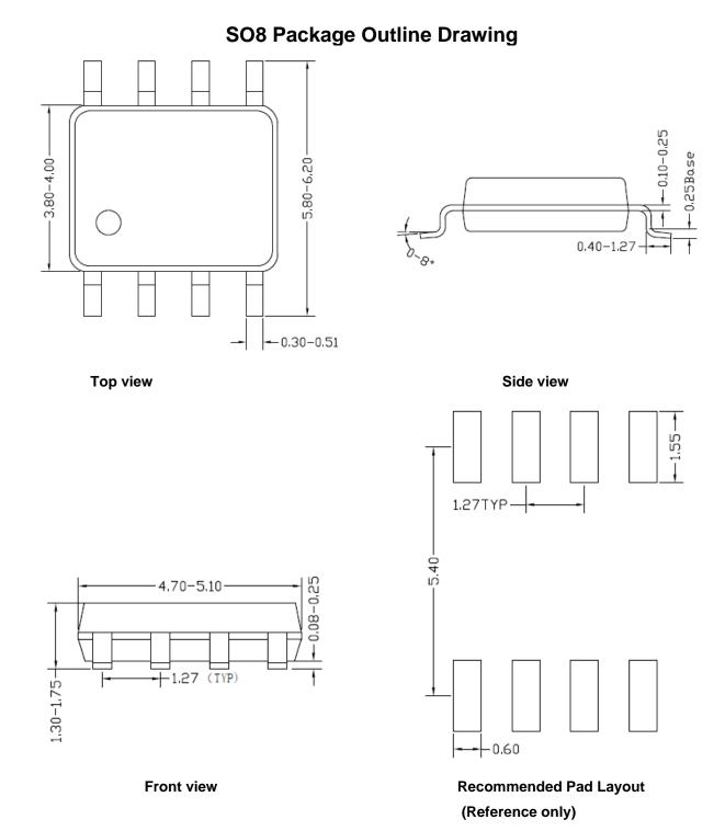
Notes: All dimension in millimeter and exclude mold flash & metal burr.
