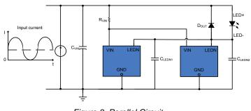
Figure 3. Parallel Circuit
