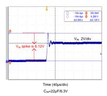
Figure 6. Voltage Spike without Suppression
