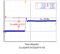
Figure 7. Voltage Spike with Suppression
