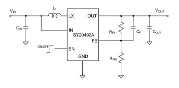
Figure 1. Schematic Diagram
