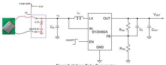
Figure 5. Voltage Spike Suppression
