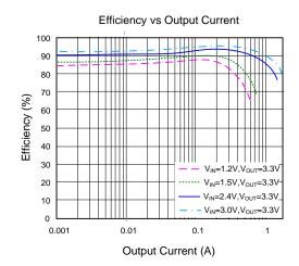
Figure 2. Efficiency vs. Load Current
