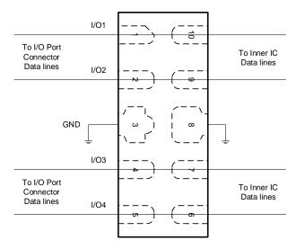
Figure 2. SY205227DVD Pin Connections in PCB
