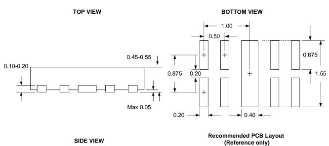
Note: All dimensions are in millimeters and exclude mold flash and metal burr.
