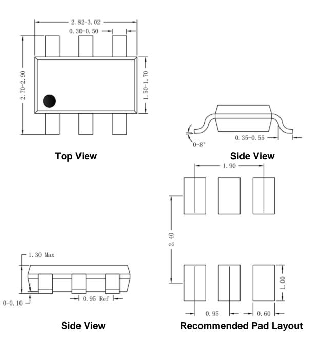
Notes: All dimension in millimeter and exclude mold flash & metal burr.
