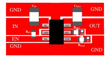
Figure 4. SY20807CABC PCB Layout Example
