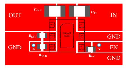
Figure 3. SY20807ZDEC PCB Layout Example
