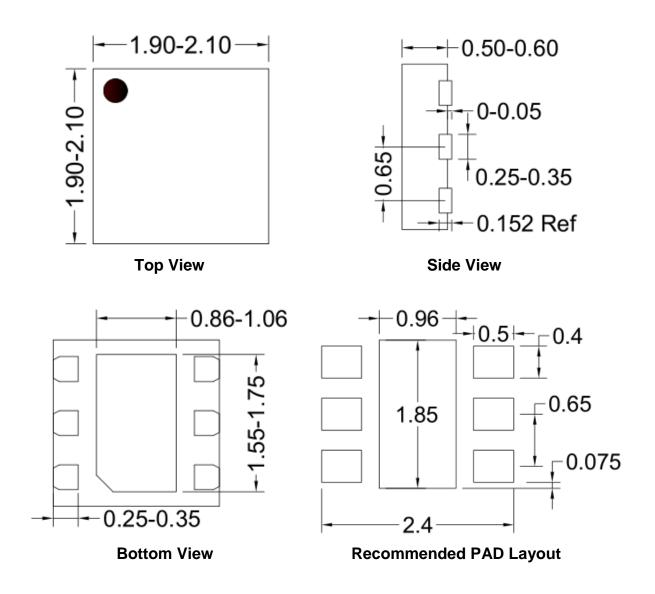
Note: All dimensions are in millimeters and exclude mold flash and metal burr.
