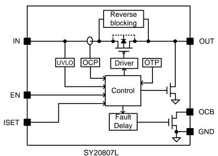
Figure 2. Block Diagram
