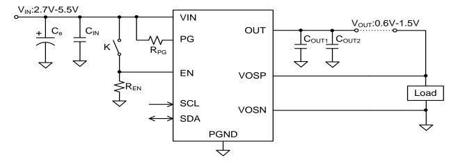
Figure 1. Schematic Diagram
