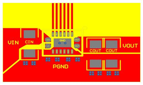
Figure 3.PCB Layout Suggestion
