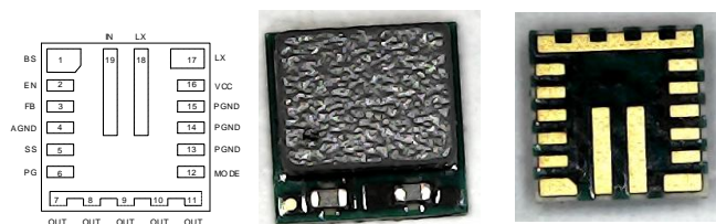
Package:MQFN 3×3-19, Height: 1.7mm max
