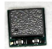
Package:MQFN3x3-19, Height: 1.5mm max
