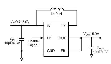
Figure 1. Schematic Diagram
