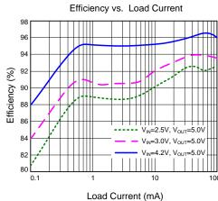
Figure 2. Efficiency vs. Load Current
