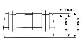
Notes: All dimensions are in millimeters. All dimensions don't include mold flash & metal burr.
