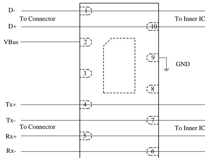
Figure 3 SYT07S05 pin connection for USB3.0 protection.
