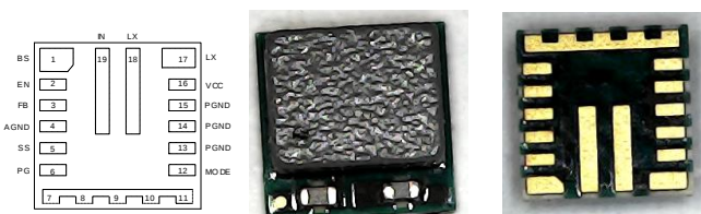
Package:MQFN 3×3-19, Height: 1.7mm max
